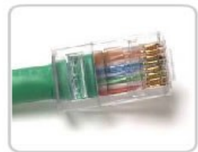
Good connector - Wires are untwisted to the extent necessary to attach the connector.
